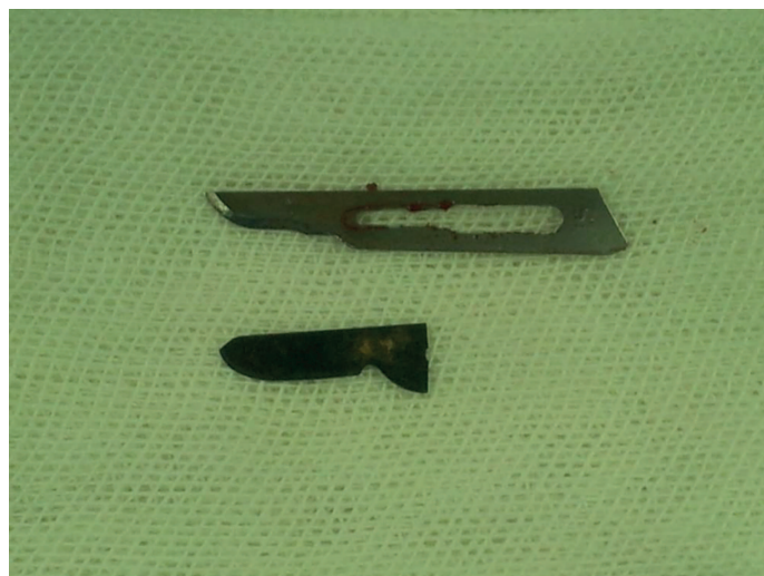
Figure 5. Comparing a surgical knife that is used in our hospital with substandard broken blade with narrow junction. Note the discoloration of the broken blade after 3 days.
