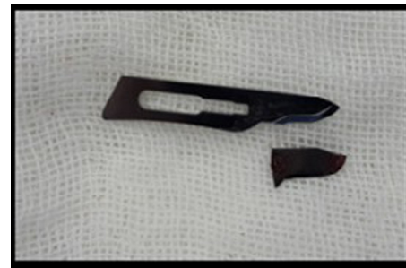
Fig. 3. Comparing a surgical knife that is used in our hospital with substandard broken blade with narrow junction. Note the discoloration of the broken blade after 3 days.
