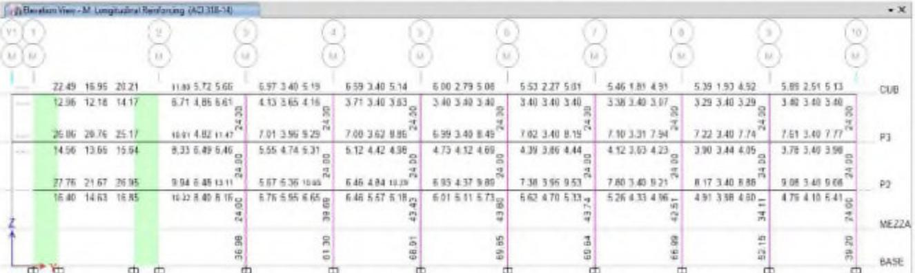
**Elevation View - Y1 Longitudinal Reinforcing (ACI 318-14)**
